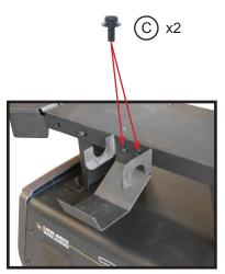
Attached torch holder to either side of the handle bracket, using 2 x C screws.
